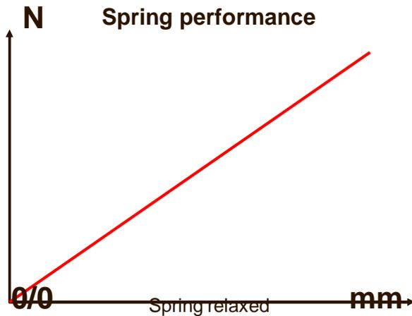
$$F_{\text{Spring}}[\text{N}] = C[\text{N/mm}] \times \Delta X[\text{mm}]$$
