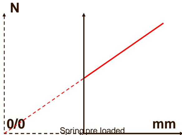
By setting a safety valve to a specific set pressure, the spring is pre loaded with force.
