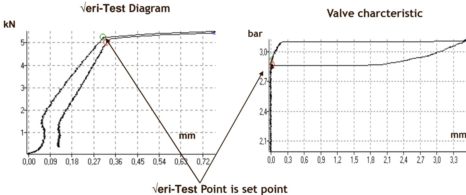
**The set point is the moment when the disk starts to lift while the valve is in an operational condition**
