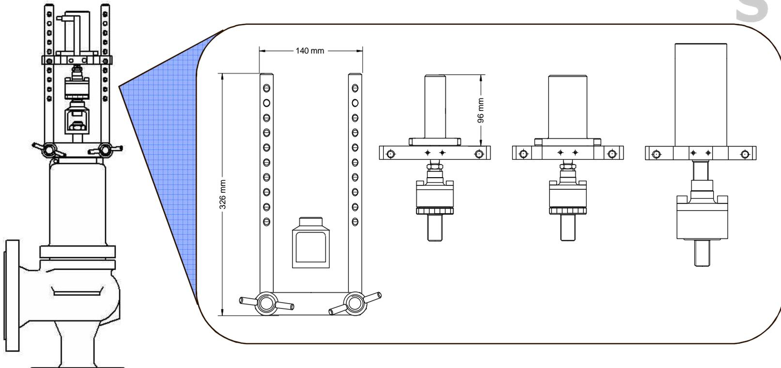
The rig consist of the metal bars and three bridges (1 kN • 10 kN • 20 kN). A bridge includes a hydraulic cylinder and a force sensor.
