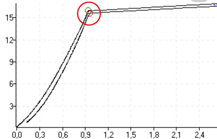
Compression of test rig and valve bonnet - NO real spindle movement !!!
